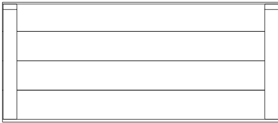
RP3 ROOF PANEL - W2A03267 (2) 1 5/8"x20 5/8"x59" (42x524x1204)
